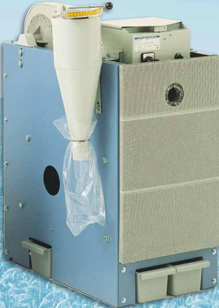
**for cleaning and grading by size as means of selecting grain for seed, malting, feed etc.**
