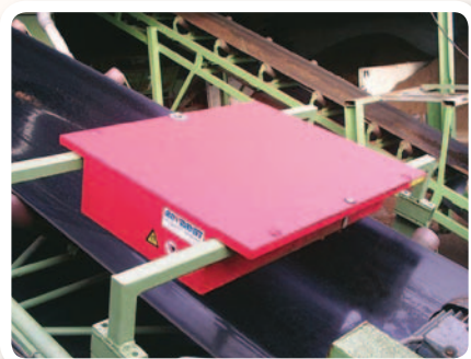
Ferrite plate magnet above belt, for removal of fe-particles from potting soil.
