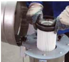
Easy maintenance thanks to hinged top cover and cartridge removal without tools
